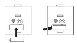
**Remarks:** The quantity, type, size and insert direction of batteries may differ depending on the model.
